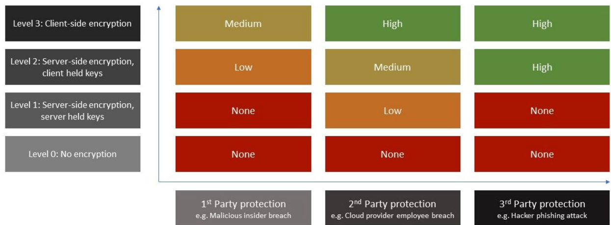
Fig. 2: What extra protections do different encryption types provide when regular access controls are breached?
